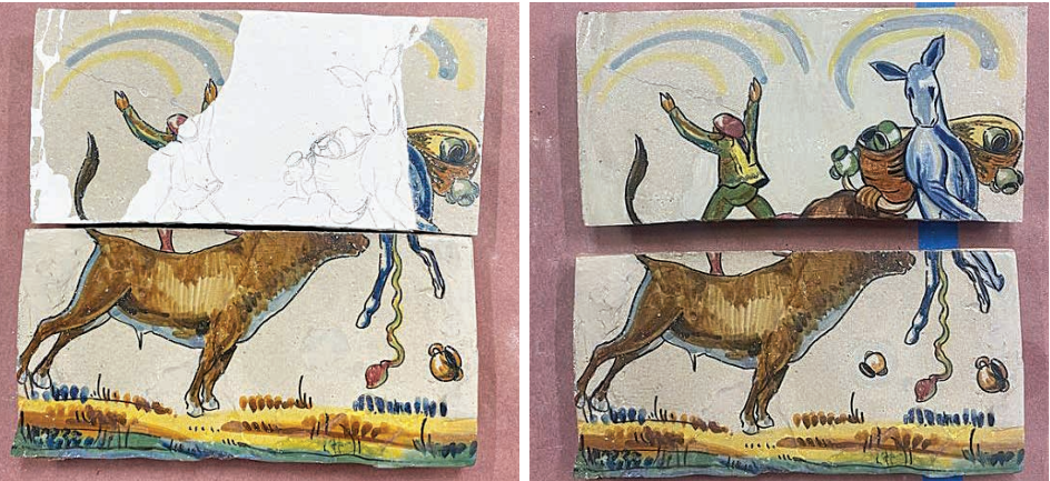
Left: The treatment process: Loose material was dry brushed off the tiles faces; the surface was washed to reduce biological growth present between the tile and glaze. Then losses on the tile faces (and backs if applicable) were filled with a conservation grade patching mortar, sanded down to match the tile’s surface, and then painted to mimic the glazing both in sheen and color. Right: Goya planter tile after treatment patching.
